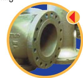
For flanged valves, use new gaskets and tighten the mounting studs evenly.
