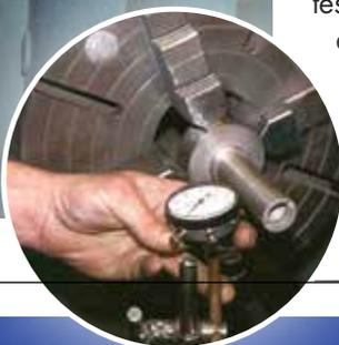
In addition to an experienced, skilled staff, North American's Service Center is equipped to handle any safety valve repair. NASVI has the specifications for nearly every safety valve ever made—allowing technicians to make repairs to exact specifications. The center has six lathes on site, so technicians can restore tolerances on existing parts in quick order. If a part cannot be restored, it can generally be replaced from our extensive parts inventory.
