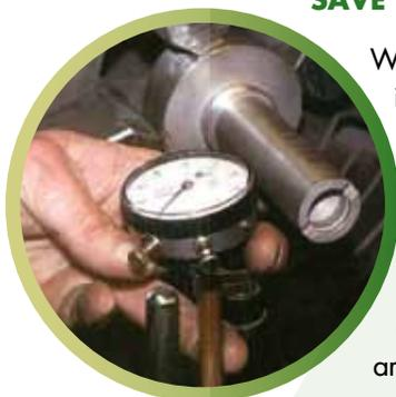
When a safety valve is remanufactured, it is completely disassembled, cleaned and inspected. Then every working part is checked for signs of wear. Everything must meet the manufacturer's tolerances to qualify for remanufacture. The castings are sand blasted and examined for defects and the flanges are refaced to a new finish.
